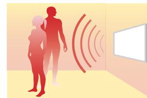
With infrared heaters the infrared radiation will be distributed uniformly in the room and absorbed by objects and walls. This creates an overall cozy and comfortable feeling of heat.
